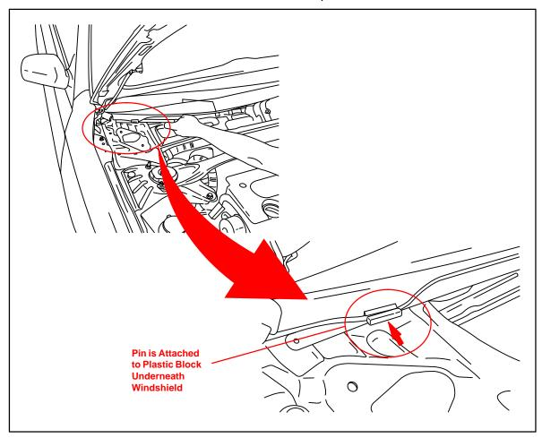
3. Use a "Mini" Hacksaw with a fine tooth 10-inch blade to cut OFF the pin portion of the glass retainer flush with the flat portion of the windshield retainer (diagram below shows the windshield retainer location to cut off the plastic pin).
