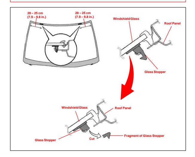
Repair Procedure (Continued) 3. Once the tip of the stopper has been removed, use a screwdriver to open a gap between the roof panel and the remainder of the plastic windshield stopper.
