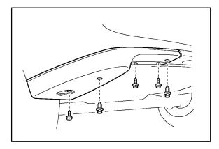
L. Install the screw to the floor under cover as shown in the illustration.
