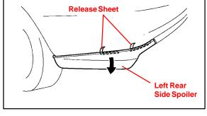
Ensure that the left rear side spoiler is attached and firmly press the adhesive tape areas of the left rear side spoiler to the rear bumper.
