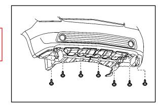
2. Install the front spoiler cover with the 7 self-tapping screws.
