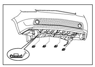
4. Install the screw grommets to the center engine under cover.
