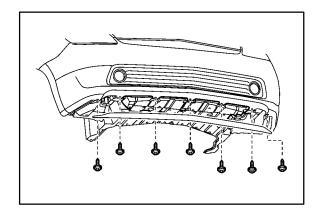
3. Install the spring nuts to the right and left engine under covers.
