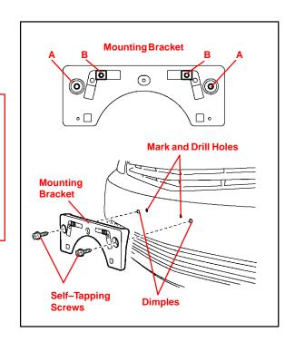
Installation Procedure (Continued) 3. Install the mounting bracket to the front bumper cover by attaching the two self-tapping screws into the dimples.
