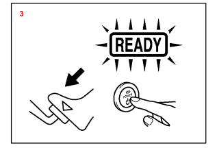
5. To stop the hybrid system (the "READY" light is OFF), make sure the "P" position switch is illuminated before pressing the "POWER" switch again. This will cause the hybrid system to stop (the "READY" light is OFF). Check that all the indicators in the meter have extinguished.
