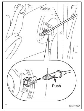
(b) Push the claw and pull out the cable.
