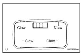
(c) Attach the 4 claws to install the room light lens.
