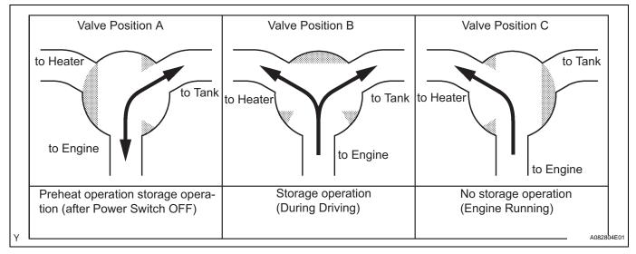
The ECM monitors the position of the water valve based on the valve position signal that is output by the water valve position sensor (potentiometer), which is coupled coaxially to the valve. The water valve effects control in three steps as indicated above, and the ECM determines the position of the valve according to the voltage of the respective step.
