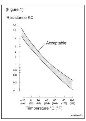
The intake air temperature (IAT) sensor, mounted on the mass air flow (MAF) meter, monitors the intake air temperature. The IAT sensor has a thermistor that varies its resistance depending on the temperature of the intake air. When the air temperature is low, the resistance in the thermistor increases. When the temperature is high, the resistance drops. The variations in resistance are reflected as voltage changes to the ECM terminal (see Figure 1).
