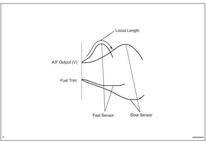
The air fuel-ratio (A/F) sensor varies its output voltage in proportion to the air-fuel ratio. Based on the output voltage, the ECM determines if the air-fuel ratio is RICH or LEAN and adjusts the stoichiometric air-fuel ratio.
