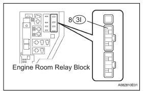
(a) Remove the integration relay from the engine room relay block.
