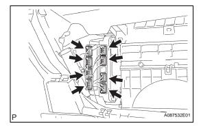
(c) Install the 3 No. 1 ECM brackets with the 6 screws.
