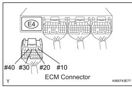
(a) Check the harness and connectors between the injector connector and ECM connector.
