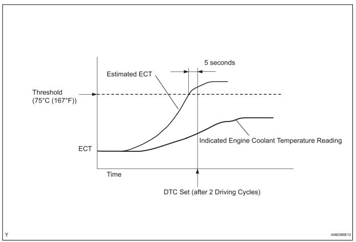
The ECM estimates the engine coolant temperature (ECT) based on engine starting temperature, engine loads and engine speed. The ECM then compares the estimated ECT with the actual ECT. When the estimated ECT reaches 75°C (167°F), the ECM check the actual ECT. If the actual ECT is less than 75°C (167°F), the ECM will interpret this as a fault in thermostat or the engine cooling system and set a DTC.
