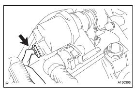
(a) Disconnect the V7 canister connector.(b) Disconnect the E7 ECM connector.
