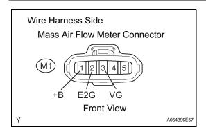
(a) Disconnect the M1 mass air flow meter connector.
