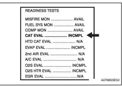
(d) Drive the vehicle according to the confirmation driving pattern. Note the state of the Readiness Tests. They will change to COMPL (complete) as the CAT evaluation monitors operate.
