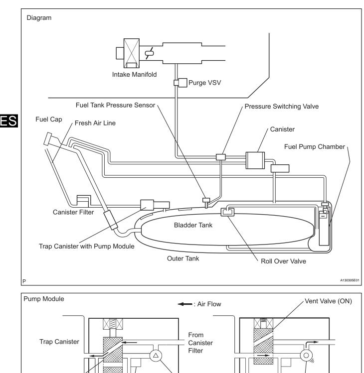
Leak Detection Pump (OFF)
