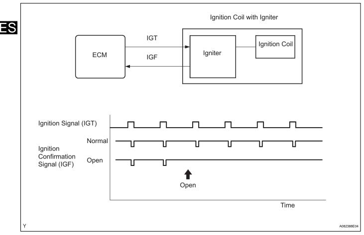
If the ECM does not receive the ignition confirmation (IGF) signal after sending the ignition (IGT) signal, the ECM interprets this as a fault in the igniter and sets a DTC.
