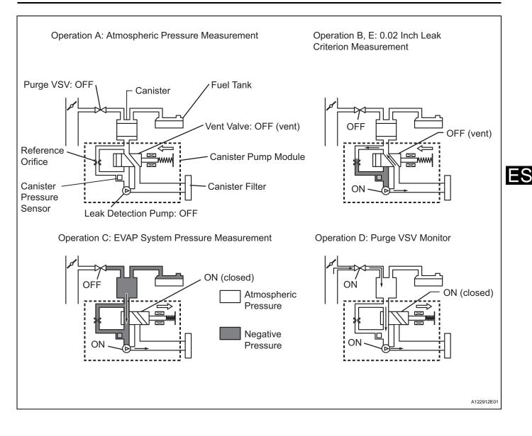
1. P2420: Vent valve stuck open (vent)
