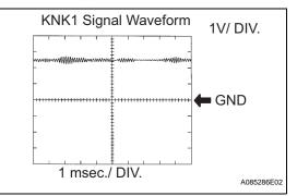
(1) After warming up, run the engine at 2,500 rpm, check the waveform between terminals KNK1 and EKNK of the ECM connector.
