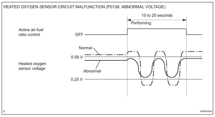
Under "active air-fuel ratio control", the ECM calculates the Oxygen Storage Capacity (OSC)\* in the catalyst by forcibly regulating the air-fuel ratio to go RICH (or LEAN).
