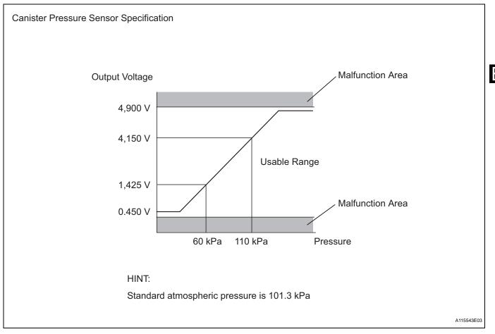
(a) DTC P0450: Canister pressure sensor voltage abnormal fluctuation
