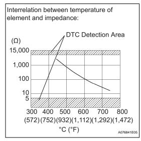
During normal feedback control of the air-fuel ratio, there are small variations in the exhaust gas oxygen concentration. In order to continuously monitor the slight variation of the signal from the oxygen sensor while the engine is running, the impedance\* of the sensor is measured by the ECM. The ECM detects that there is malfunction in the sensor when the measured impedance deviates from the standard range. \*: The effective resistance in an alternating current electrical circuit. HINT:
