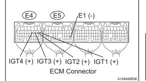
(a) Measure the voltage between the applicable terminals of the E4 and E5 ECM connectors when the engine is cranked.
