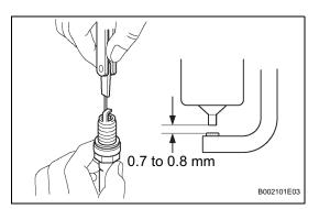
(c) Check the spark plug type. Recommended spark plug:
