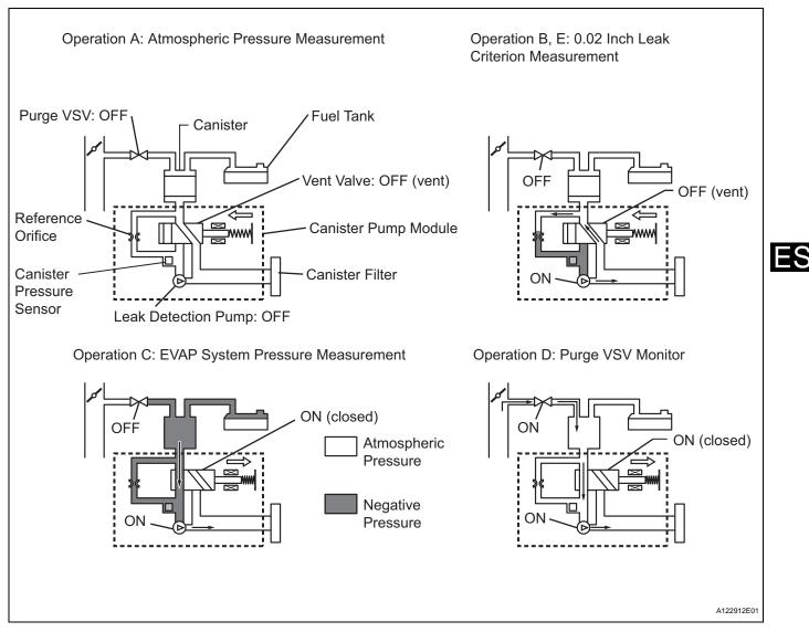
In sequences B and E, the leak detection pump creates negative pressure (vacuum) through the reference orifice. If the pressure is lower than 724 mmHg-a, higher than 752 mmHg-a, is not saturated and the pressure difference at sequences B and E is large, the ECM interprets this as a clog malfunction in the reference orifice, and stops the EVAP system monitor. The ECM then illuminates the MIL and sets the DTC (2 trip detection logic).
