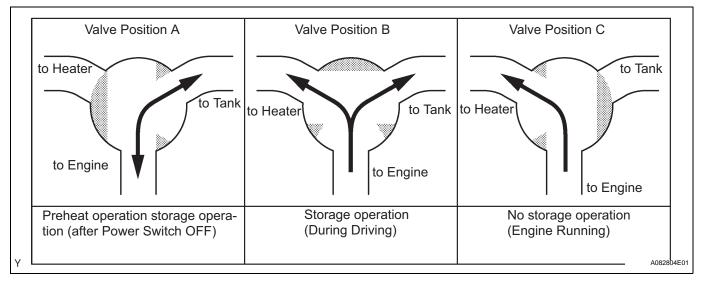
A potentiometer is provided in the coolant heat storage (CHS) system. The ECM uses the valve position signal output by the water valve for effecting control that is appropriate for the operating condition of the engine. The water valve effects control in three steps as indicated below, and the ECM determines the position of the valve according to the voltage of the respective step.
