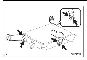
(e) Remove the 6 screws and 3 No. 1 ECM brackets.
