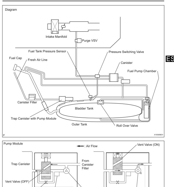
Leak Detection Pump (OFF)
