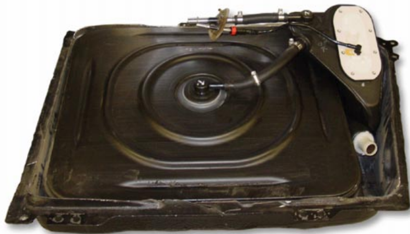
Tank cut opened to show bladder
