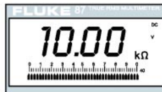
Display showing 10 Kilo-ohms
