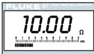
Display showing 10 Ohms
