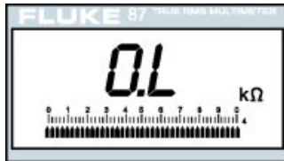
Display showing over-limit
