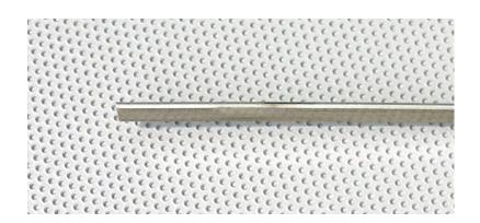
This thin &, curved piece of metal is the "spine" of the wiper-blade. It provides rigidity, to keep the entire assembly flat against the windshield yet flexible to bend along the contour of the glass as the wiper moves.
