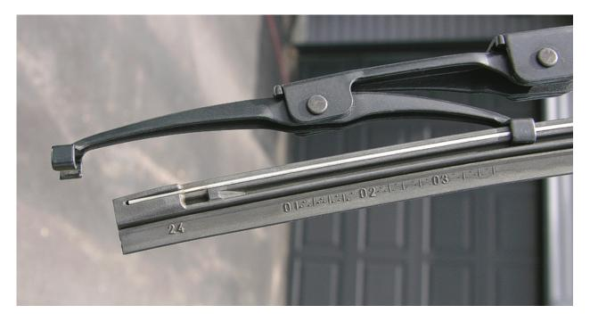
Once wiper-blade is loose, you can pull it out entire to replace the rubber blade and reinsert the metal spine.
