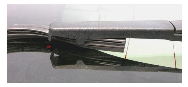
The front wipers do not require a grip to be removed. They can be lifted (as shown below) simply by just pulling up on each of them individually.
