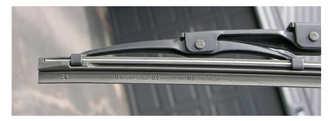
Above is an extreme close-up of the front wiper-blade. Notice (near the "24" on the photo) how it is locked into place with a metal clamp that reaches into the rubber itself.
