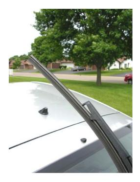
To remove the blade from the wiper, just bend it a little in the middle until it gives enough to clear the stopper at the end of the plastic housing.
