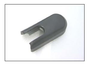
On the previous page, you'll see the rear wiper as it usually looks. At the base of it, notice the plastic clamp (close-up shown to the right). Firmly grab that clamp with your hand, pulling upward. The two edges will give, allowing you to remove it entirely.
