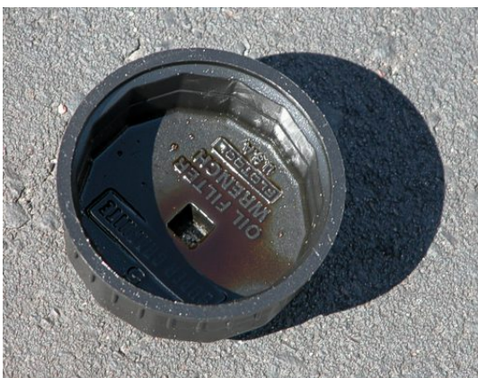
Filter Wrench Checker Part: 32100-10605
