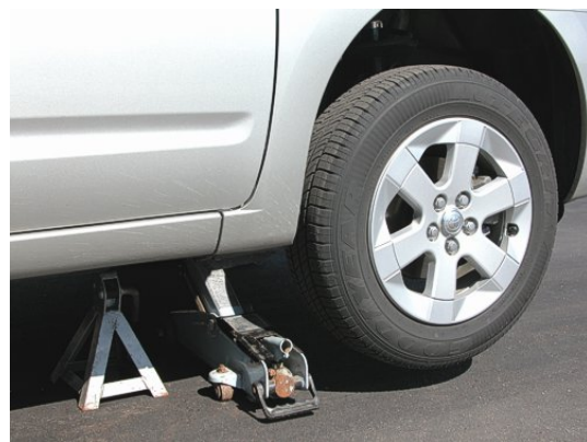
After lifting, with stand support.
