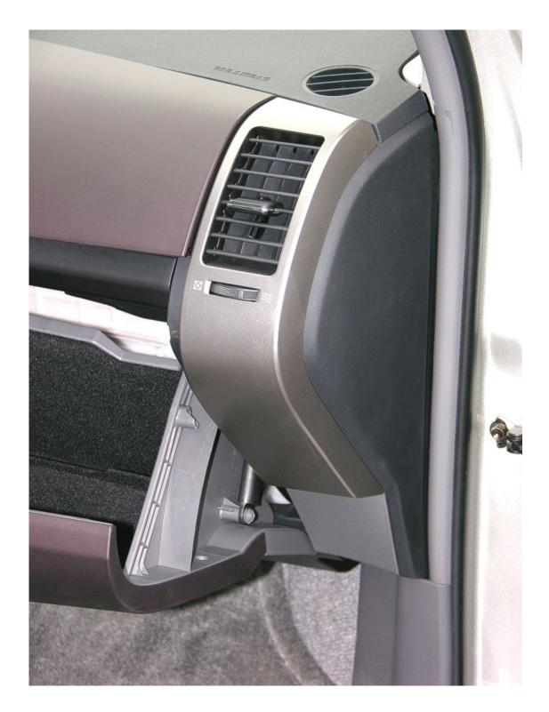
Back on the right side, notice how there is an attached arm preventing the glove-box from dropping to the floor. This is a plastic shock-absorber that dampens (makes softer) movement when opening & closing the glove-box.
