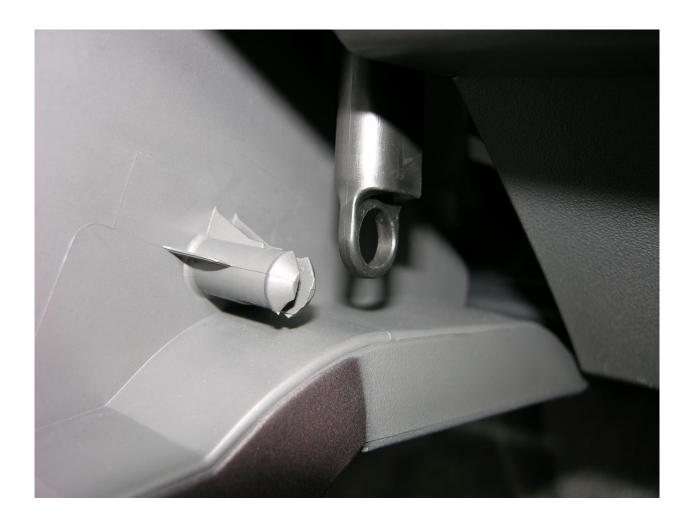
Above is an extreme close-up of the dampener and the arm in which it attaches.
