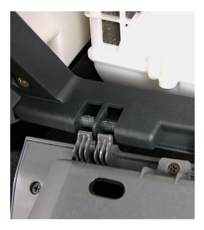
Once you have properly refitted the glove-box, reverse the process you performed earlier. Connect the dampener to the glove-box, by pushing the eye into the gripping arm. Then push on the outside of the glove-box to make the flexible plastic bend allowing that catch on each side to slip behind the stops. At that point, you are done!
