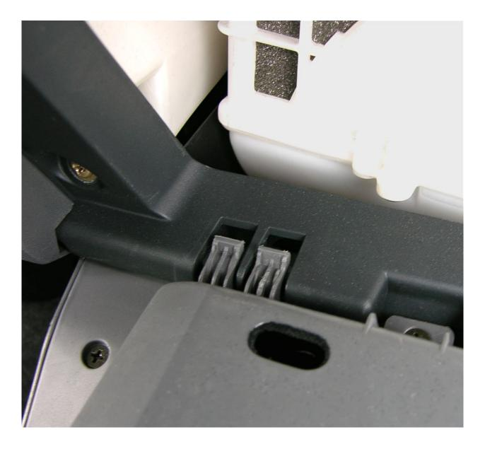
This extreme close-up shows what the hinges at the base of the glove-box are supposed to look like when attached properly. Unfortunately, the weight of the glove-box hanging upside-down is enough to pull the hinges out, as shown on the next page.
