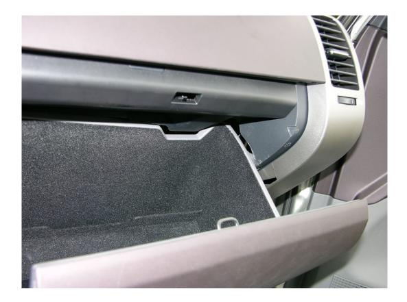
Above is the right side of the glove-box. Begin the process to reveal the hepa filter behind it by simply pulling inward with your hand. No tool is required. The flexible plastic will bend allowing the catch to be bypassed.
