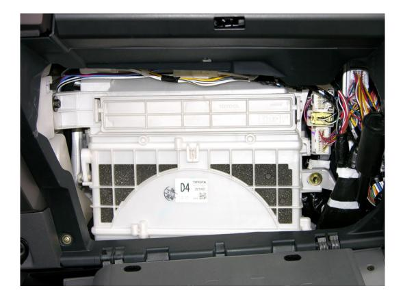
Above is the plastic box in which the hepa filter and air-conditioner fan is located. To remove the hepa filter, all you have to do is pull on the two tabs at the top of the white area, on the left & right side. An inch tall horizontal cartridge will easily slide out.
