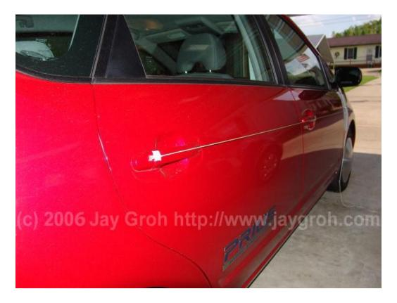
String it all the way to the front of the car to where the bottom of the finder, the top part of the bumper, and the light meet. Make sure this string is straight!
