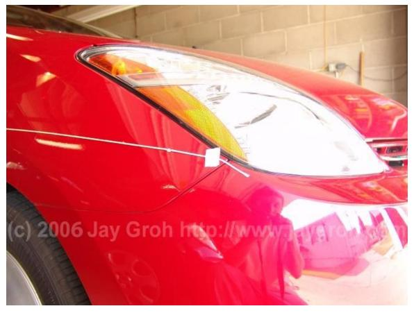
3. Put another piece of string where the front A pillar meets the finder. Get it in between the crack and pull it straight down to the bottom edge of the wheel well. Make sure this string is straight!
