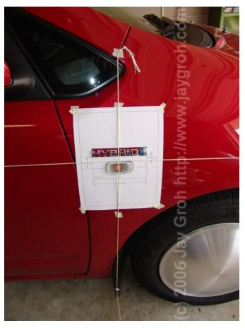
4. Place the template behind the string and line up points A B C and D indicated on the template. A and B are at the top and bottom. C and D are left and right. When you get your strings centered with the lines A B C and D tape it and stand back and see if that where you want it. Make things the way YOU want and when your done you can start cutting away.
