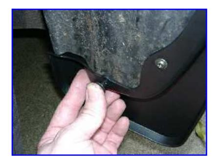
Once the hole is drilled and you have cleaned off the plastic bits, insert the pushclip provided.
