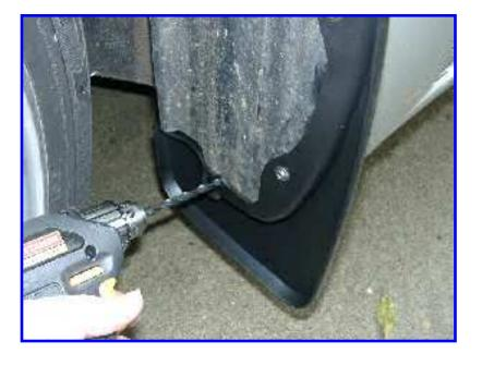
Next, drill a 6mm hole through the plastic wheelwell shield. If you don't have a 6mm (0.23622") bit, you can use:
