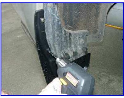
Then loosely screw in the top screw to help hold the top of the splashguard in place while I drilled the second hole. Add the springclip for that hole, hold the splashguard tight to the fender, and tighten the 2 screws down.
