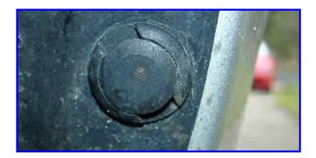
You first need to remove the bottom two pushclips. Note the 2 slots on the base of the clips.
