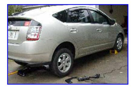
First you need to block the front wheels (Although the vehicle is in park, I still urge you to block the wheels). Next, loosen the lug nuts on the rear tires slightly. I used a 4-way lug wrench. The lug nuts are 21mm. Then jack up the car.
