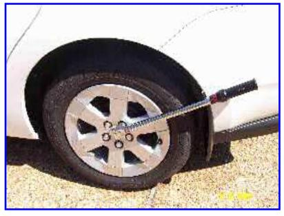
Finally, torque your lug nuts down (76 ft-lb). If you don't have a torque wrench, make sure the lug nuts are tight and try to ensure each one is only as tight as the others. Use a "star" pattern when tightening.
