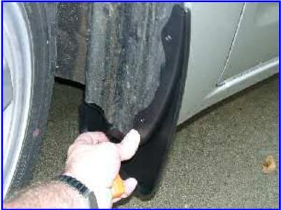
Next, line up the splashguard with the two holes where the push clips used to be, and insert two metal screws into the holes and spring clips. As you tighten down the two screws, gently push the splashguard against the car so that it makes a tight fit.
