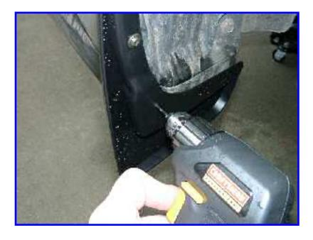
For the third screw, use a 2.5mm bit and drill the bottom hole, then insert the metal screw (*Do not, do not, do NOT* drill a 6mm/½" hole here, it will be way too big!!!). If you don't have a 2.5mm (0.0984") bit, you can use:
