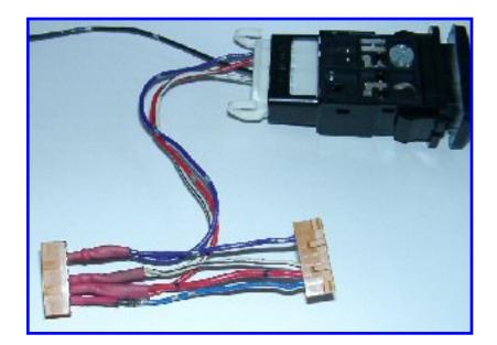
Here's the finished Y-harness, ready to be installed. You can wrap the wires with electrical tape or tubing harvested from a junkyard car, if you want to make it look neater. Note the black wire at top is the one that will be going to the ECU later.
