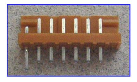
This 8-pin plug will be used to connect to the factory dashlight dimmer plug. Unfortunately, I do not have a part number for this plug yet. Since you are only using 4 of the pins, it is best to remove the others to avoid confusion. Simply press them out from the front, as shown.
