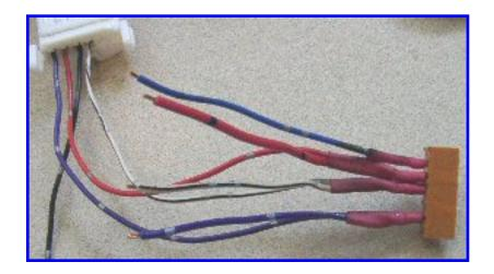
Heat the heatshrink tubing to shrink it down. Strip the other ends of the 4 jumper wires. You are only going to be stripping off about 1/16" - *very* little insulation.
