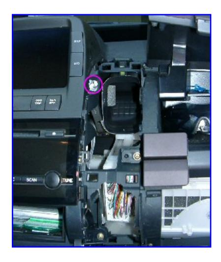
Remove the passenger side center vent panel by pulling at the top and bottom. Remove the MFD bolts on each side, as circled (10mm).
