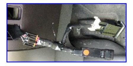
Wiretie the plugs together...but *not* as shown. The wiretie goes over the release tab on the dimmer plug in this picture. Then depress the tabs for the EV button blockoff plate and push it out from behind. *Make sure to save this blockoff plate in case you need it in the future*.
