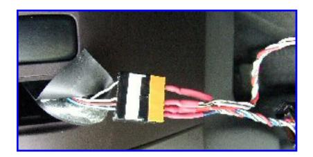
Remove the driver's side vent panel by pulling on the top and bottom. Reach behind the dimmer switch, find the tabs holding it to the dash, and depress them. Push the dimmer out and unplug it.
