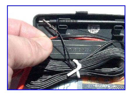
If you have a DVM (*highly* recommended if you do any work on cars, the one pictured is only about \$20 from Radio Shack, and is a pocket folding DVM), test continuity from the terminal to the other end of the wire...
