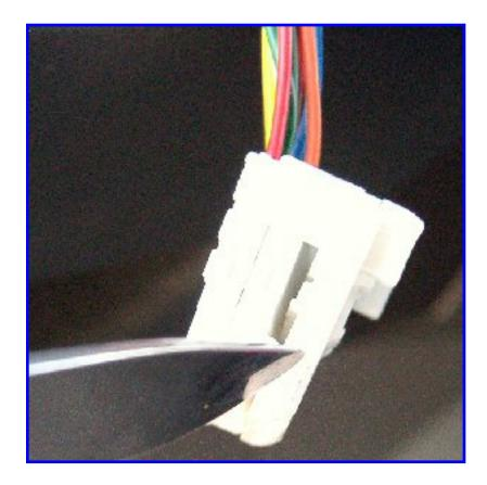
Pry the top set of smaller tabs loose as shown, and the top of the plug should just fall off.
