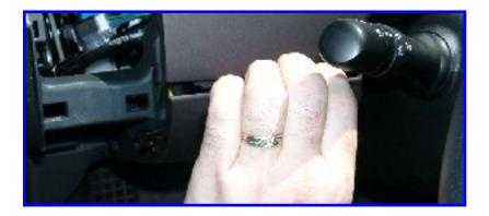
Pull along the lower panel until you pop the clip near the steering column loose.
