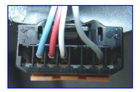
The back of the factory dimmer plug, showing the factory colors and their placement in the available 8 sockets.
