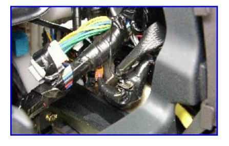
Tuck the Y-harness out of the way under the factory harnesses, so it doesn't interfere with the vent panel when it is replaced, or rattle against anything. You can see the ECU EV wire in front of the dash wiring here, waiting to be spliced to a longer wire to run to the ECU to actuate EV mode.
