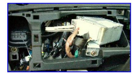
Route the splitloom (with the EVb wire inside) from the glovebox area, behind the MFD, behind the ECU shown here (above the steering wheel, and over to the EV button area, as shown in this and previous pictures.
