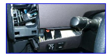
Once you have the lower panel popped out partially as shown, you can start removing the upper panel.
