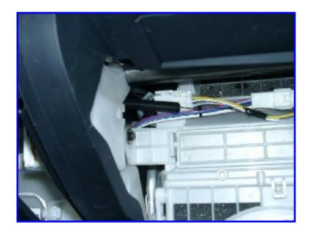
At this point, you can run the wire from the glovebox area over to the button in many ways, including taping it to a straightened coathanger and pushing it behind the MultiFunction Display (MFD). I'm Mr. Overkill, so I disassembled the dash a good bit and ran splitloom tubing, as shown in the upper left corner of the glovebox opening.
