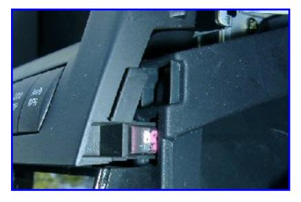
Pull back on the bottom corners of the MFD, above the radio, to release the clips shown.
