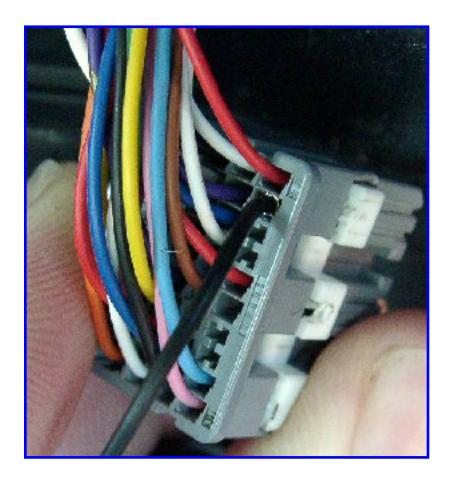
Once it is in far enough that you can't push on the bayonets, push on the wire retaining tabs. Push until the end of the terminal is slightly below the level of the plug, as shown. Then push the white terminal retainer back down into the plug, and plug it back into the ECU.
