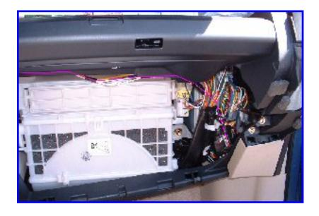
Run the EVb wire up along the stock wiring harness in the route shown, using wireties every few inches to make sure the wire is out of the way and secure.
