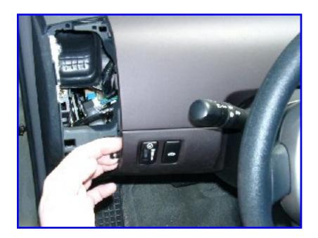
Start back over at the EV button area. Pull back on the lower dash panel as shown. Until the tab nearest your fingers on the lower panel pops loose.
