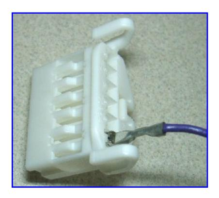
Insert the factory wires/terminals into the plug. These wires were obtained from junkyards, they come from 87-up Toyotas, I believe. Check the stereo plugs, and some of the plugs near and plugging into the fusebox, and ones behind the glovebox. Note the fins on the terminals that form-fit to the plug.
