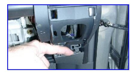
Remove the right vent by pulling at the top and bottom, making sure the top glovebox is open so one of the vent retaining clips can come loose. Then remove the pictured lower panel by pulling the top loose, then pulling it toward you.
