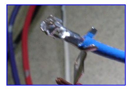
Fold the other flap over, make sure both flaps are compressed well, then solder quickly, with just enough solder to fill that junction, and no more.
