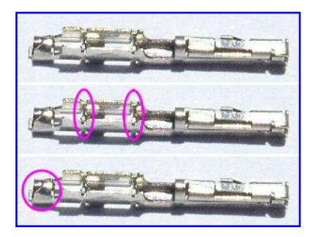
Three views of the plug, top so you can see it with no markup. In the middle, I have circled the bayonets in the terminal that cut through the wire insulation and make contact with the wire core. At the bottom, I have circled the tabs that you bend around the wire insulation to help hold the wire in place.
