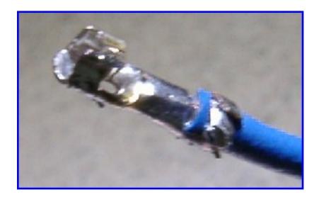
Trim the excess metal from the terminal, and fold the flaps down over the wire insulation, crimping them down tightly. You need them compressed as much as possible to properly fit the terminals into the plug.
