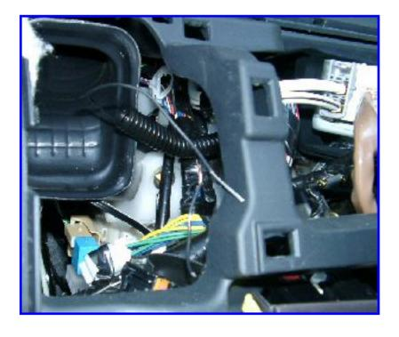
Put some heatshrink tubing over the EVb wire and wrap it to the leftover wire from the Y-harness. Temporarily plug the Power button and MFD back in, Power up, get the MFD to the Climate screen as soon as possible, and test the EV button. If it switches to the Energy screen, Power down, solder the EVb wires together, shrink the heatshrink tubing over the solder junction, and put the dash back together.
