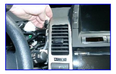
Pull out on the top of the shifter vent panel, then the bottom, then slide it upwards to get it out from under the lower dash panel.
