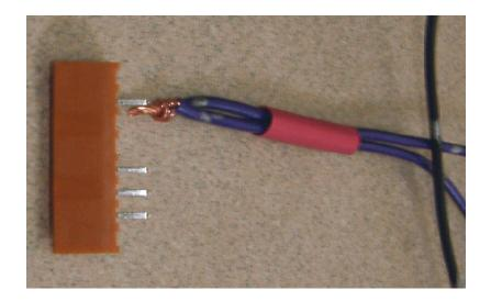
Make sure the wrapped wire does not extend all the way to the end of the EV button wire. Place some heatshrink tubing over both wires (or use tape later, but heatshrink is much better). Repeat for wires 2 and 4 from the EV button plug.
