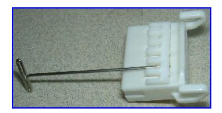
Start by using a pin or small screwdriver to remove the plug's terminal retaining bracket. If you look carefully at the plug, you will see that some of the notches surrounding the retainer are beveled. Pry within those notches. Work across each one, lifting the retainer a bit at a time, until it is completely loose.
