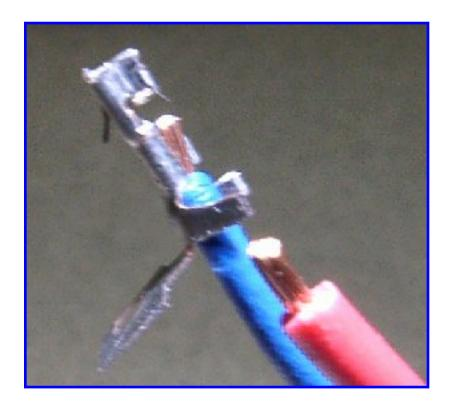
This is why you are stripping off very little. You only want enough wire exposed to fill the first crimp section of these terminals for the female 8-pin plug. Fold one flap over the exposed wire as shown.
