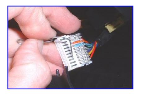
Use a paperclip, jeweler's screwdriver, etc, and depress the tab on a terminal that does not have a wire installed into it, and push it out of the plug. You can pull several and put the steering column back together, or you can do what I did, which is pull one terminal, install it in the ECU plug, and after verifying it works, then put this plug and the steering column back together.
