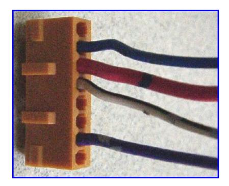
Attach all 4 terminals, then slide the wires into the plug. Again, if you are matching the factory dimmer colors, they will be grey, red, black, and white/black. I used purple in place of grey for this harness.
