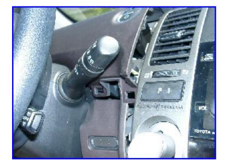
Then lift the upper panel upwards and towards you, unplug the Power button from it, and set it aside.
