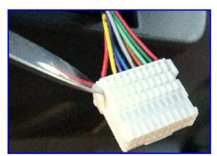
it doesn't need to be out much to work on it). Pry the larger tabs on the plug loose as shown.
