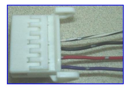
Insert the retainer, pushing it down until it locks in place.
