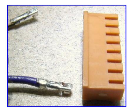
The bottom of the terminals has a tab that locks into the slots in the plug.
