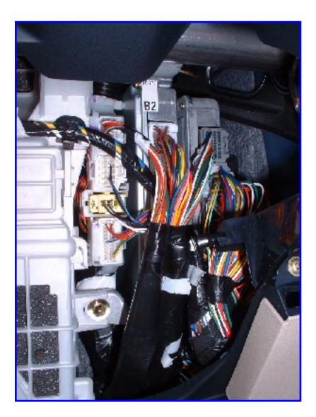
Behind the vent panel area, to the right of the gloveboxes, you'll see a ton of wiring, and several ECUs. We need the far right ECU with the grey plugs.
