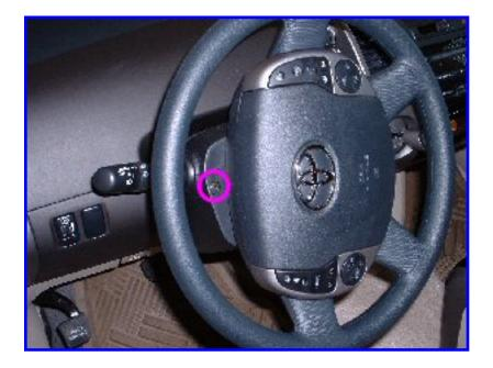
Turn the wheel to the left and remove this screw.
