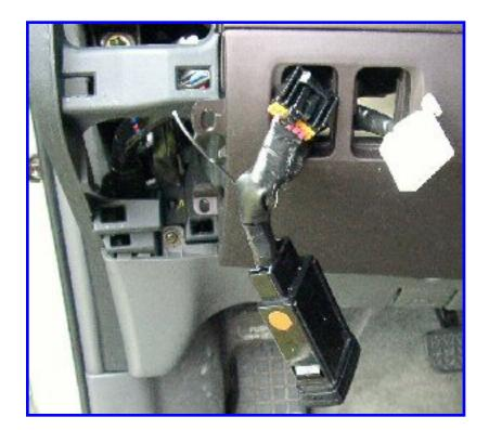
It's better to run the wiretie under the release tab, as shown here, to avoid pressure on it if you remove this mod in the future. Because the Y-harness plug is so hard to get onto the dimmer, I did not want to remove it, so I pulled the vent panel out to easily access the back side of this area, pulled the EV button plug through the dimmer hole, and pushed it back out the EV button hole.
