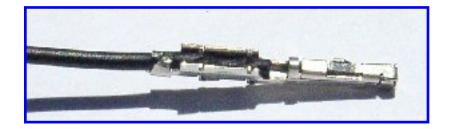
...and if it tests out OK, bend the wire retaining tabs down over the wire.
