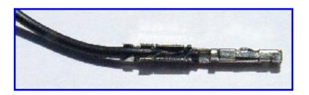
Bend the wire retaining tabs open, place the wire into the terminal as shown, and press it down into the terminal with a small flatblade screwdriver.
