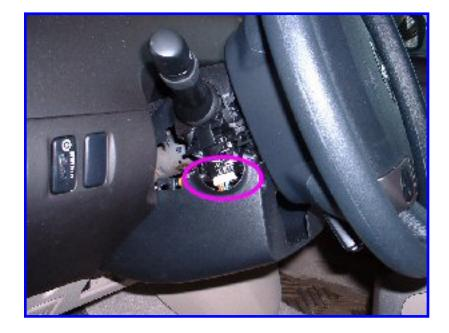
Pull down on the lower half of the cover. You may have to wiggle it around and shift it from side to side while pulling down in order to release the internal tabs holding it to the top half. The plug you need to access is circled.
