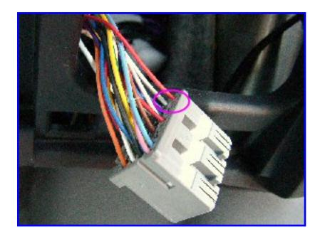
Unplug H14, and pull it out through the opening that was covered by the small bottom panel. If you orient the plug as shown, pin 27 is circled, next to the top red wire.
