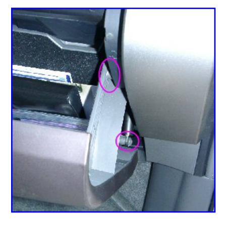
Now that you have the wire ready to insert into the ECU plug, it's time to get to the ECU. Open the top and bottom gloveboxes. On the bottom one, pull the sides of the glovebox in at the retaining tabs (upper cirle) at each side, and pull the glovebox down. Then pull the piston from the pin (lower circle), and pull the glovebox toward the seat to remove it.
