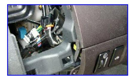
Plug the EV button in, and push the dimmer and EV button into their holes. You can see the dimmer plug and Y-harness in the middle top of the picture.
