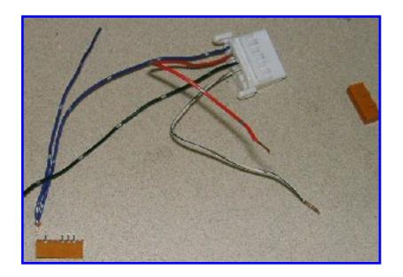
Trim wires 1, 2, and 4 to the same length. Strip about &3/8" of the insulation from the end of all 4 wires. Cut 3 pieces of jumper wire at least 3" long, strip about ¼" insulation from the ends. Wrap the stripped end of the jumper wire around the end of the EV button wire 1, as shown.
