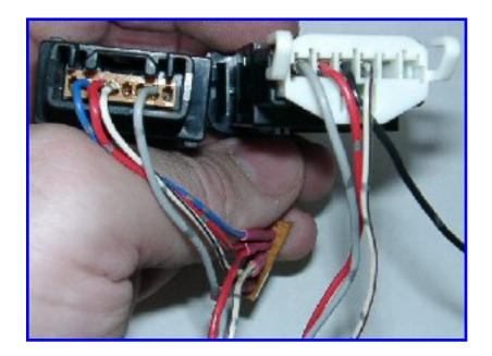
The harness inserted in the dimmer and EV button. Note that this harness *does* have the grey wire.
