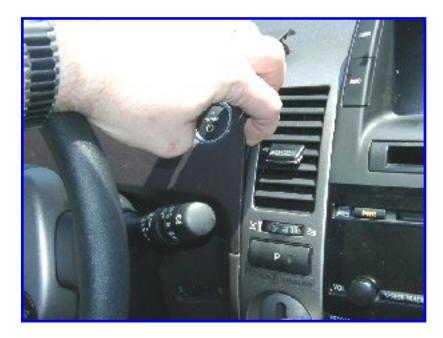
Pull on the right side of the upper panel in order to shift the lower panel out a bit.
