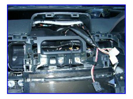
Pull the MFD back and up, disconnect all plugs, and set it aside. Here you can see the splitloom tubing I routed from one side of the dash to the other (center, black loom, behind dash structure).
