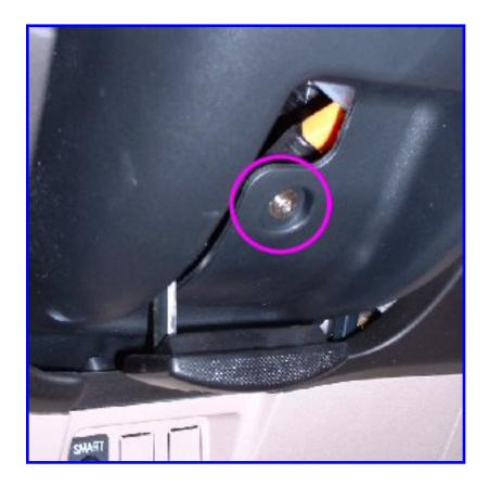
Now it's time to harvest a terminal from the highbeam flasher plug. Remove the circled screw on the underside of the steering column cover.
