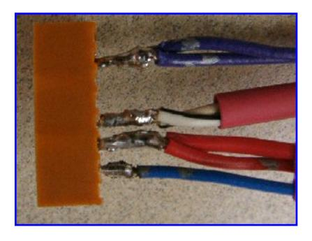
Tin the pins on the 8-pin plug (use a low heat soldering iron, or do it very quickly). Tin the ends of the wires, leaving excess solder on them. Keep them hot, then touch them to the pins on the 8-pin plug. You want to do these solder joints very quickly, or you will melt the pins loose in the plug. Note that the bottom pin has a single wire on it.
