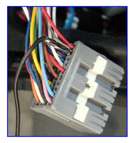
Insert the terminal/wire you assembled *in the orientation shown*. Get it into the plug by placing a small screwdriver against the bayonet blades and pushing.
